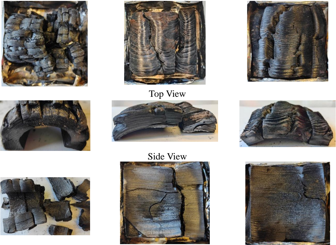
(a) Beech (b) Pine (c) Spruce Figure 15 : Top, Side and Rear Side view of the Residues of different wood
