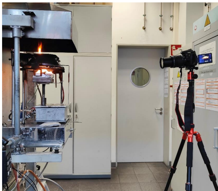
Figure 3 : Cone Calorimeter test set up.
