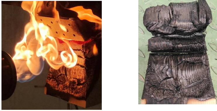
Figure 32: Burning process and the residue of the 42mm Spruce wood (Half Lap Joint).
