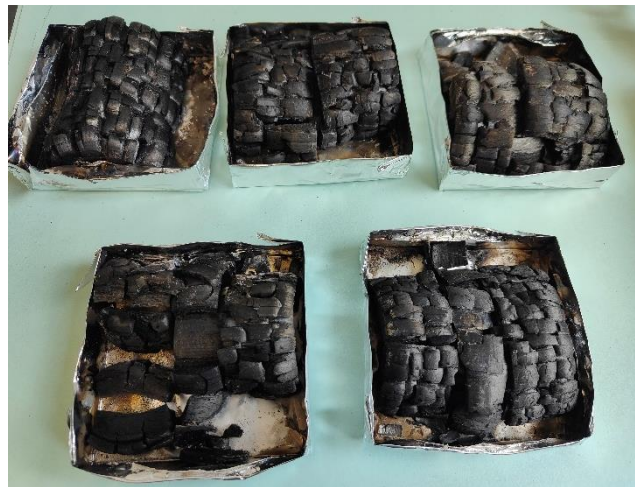
Figure 23 : Residues of the burned hard wood under 35 \text{ kW/m}^2 (Beech)
