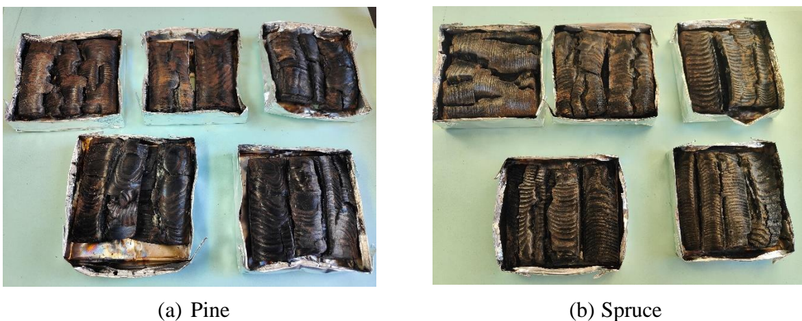
Figure 21 : Residues of the burned soft wood under 35 kW/m 2 (a) Pine, (b) Spruce
