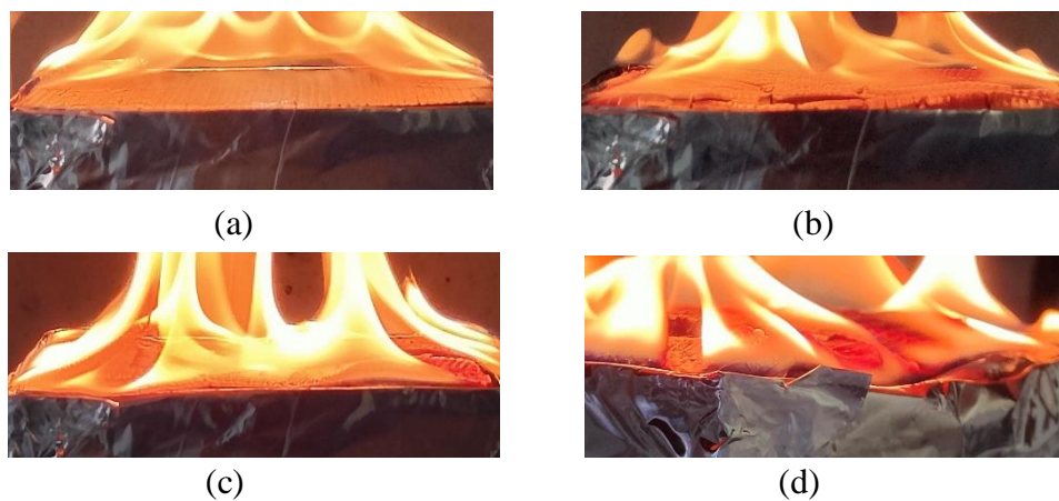
Figure 12 ; Burning of Spruce Wood (a) Beginning of the test 40 sec, (b) 300 sec where the char layer formed in the upper layer, (c) 660 sec where the specimen shrunken in the middle, (d) 1200 sec where specimen swelled in different parts.
