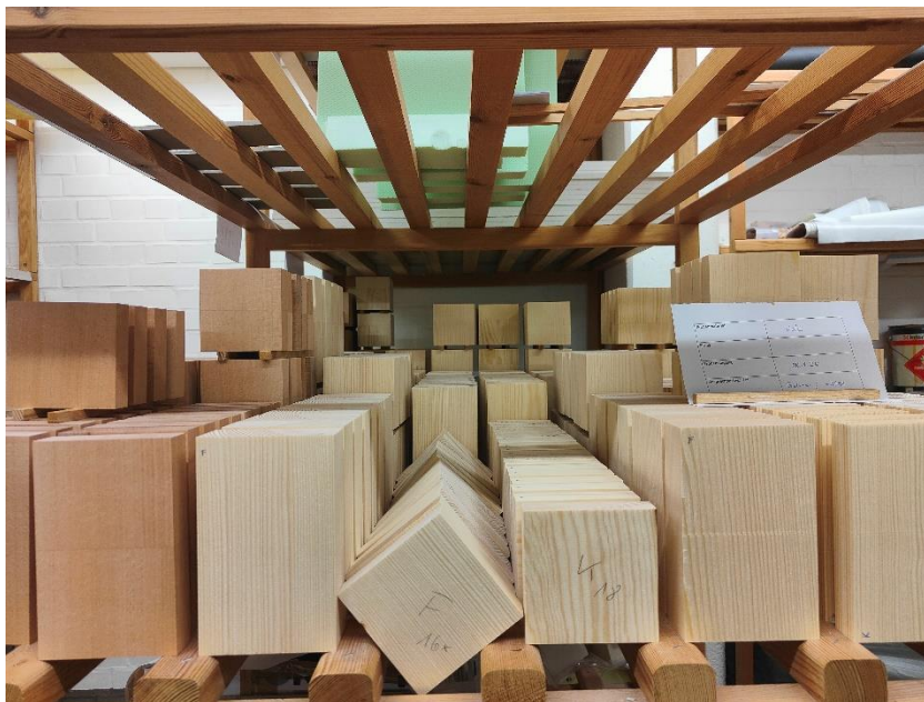
Figure 2 : Samples Stored under conditioned temperature and humidity.
