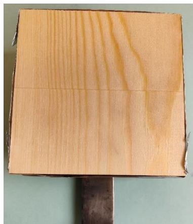
Figure 5 : Sample Preparation for Cone Calorimeter Test
