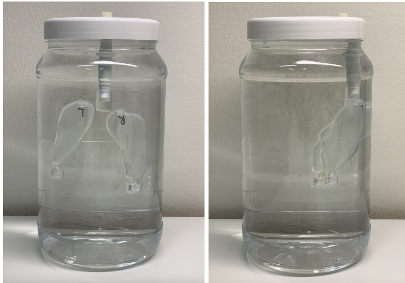
Figure 3.4: The total phantom used for the scintigraphic scans. A thyroid phantom of model A3 is placed inside the cylindrical phantom, representing the neck of a patient.
