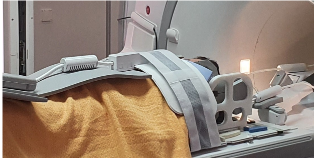
Figure 8: The setup of a healthy volunteer, showing the flex coils attached to either side of the head and across the body and neck.
