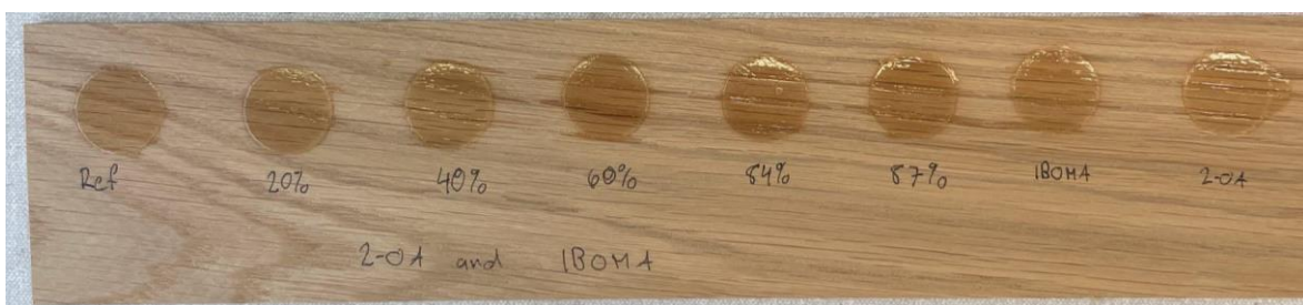
Figure 15. From left to right: 1. Reference with MMA/BA. 2. 10 wt% of each IBOMA/2OA. 3. 20 wt% of each IBOMA/2OA. 4. 40 wt% of each IBOMA/2OA. 5. 40 wt% IBOMA, 44 wt% 2OA. 6. 43 wt% IBOMA, 44 wt% 2OA. 7. IBOMA/BA. 8. 2OA/MMA.
