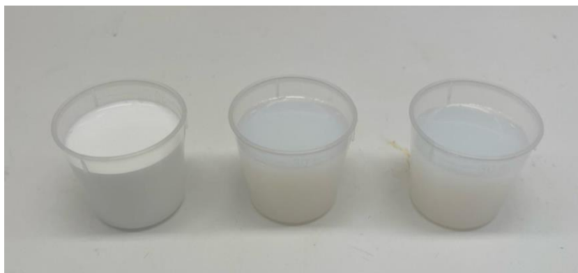
Figure 12. Color differences of the dispersion (from left to right): 5wt% cyclodextrin, 1wt% cyclodextrin and no cyclodextrin.
