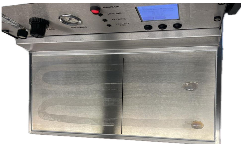
Figure 11. Picture illustrating how the MFFT was determined. Black line represents the temperature where the latest crack could be seen= MFFT. Picture is viewed from the above.
