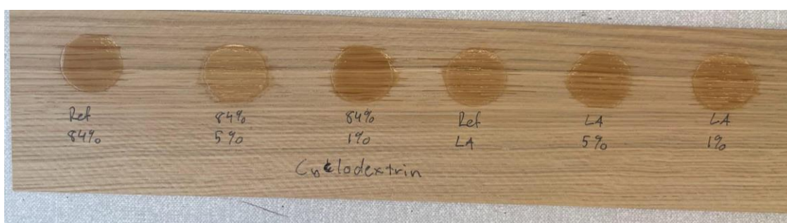
Figure 17. From left to right: 1. IBOMA/2OA. 2. 5 wt% cyclodextrin IBOMA/2OA. 3. 1 wt% cyclodextrin IBOMA/2OA. 4. LA/MMA. 5. 5 wt% cyclodextrin LA/MMA. 6. 1 wt% cyclodextrin LA/MMA.
