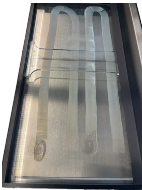
Figure 13. MFFT of the dispersion containing 5 wt% cyclodextrin, cracks all over.
