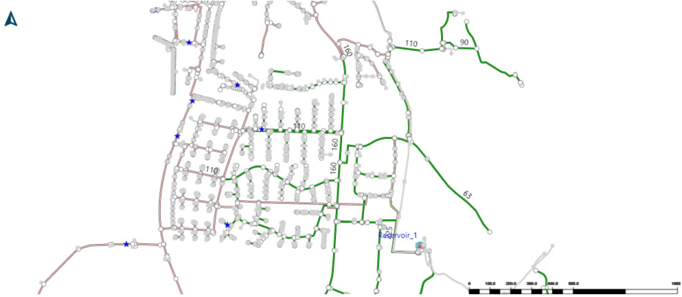
Figure 4.10. Emitters scattered to simulate pipe leakage
