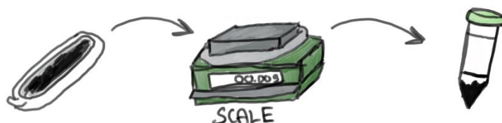
Figure 13. The activated sludge biochar from the pyrolyser's boat being weighed and transferred to a container.
