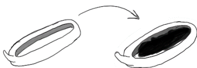
Figure 12. The boat in which the biochar was loaded and put into the pyrolyser.
