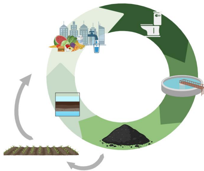
Figure 5. A Schematic sketch of the circular usage of biochar. It begins at the wastewater treatment steps where biochar is obtained from sludge. Biochar can then be reused for wastewater treatment for an adsorption-step or applied in agricultural uses. By contributing to food and clean water, the cycle continues as cities contribute to more wastewater which will re-enter the cycle.
