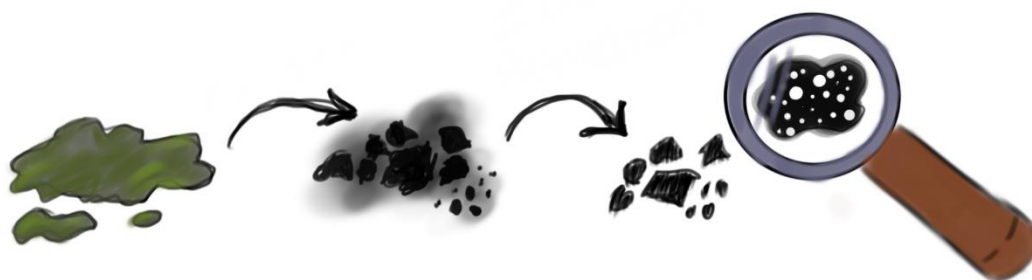
Figure 6. Sewage sludge is carbonized into biochar. Biochar is then activated to increase the porosity, as shown in the magnifying glass.
