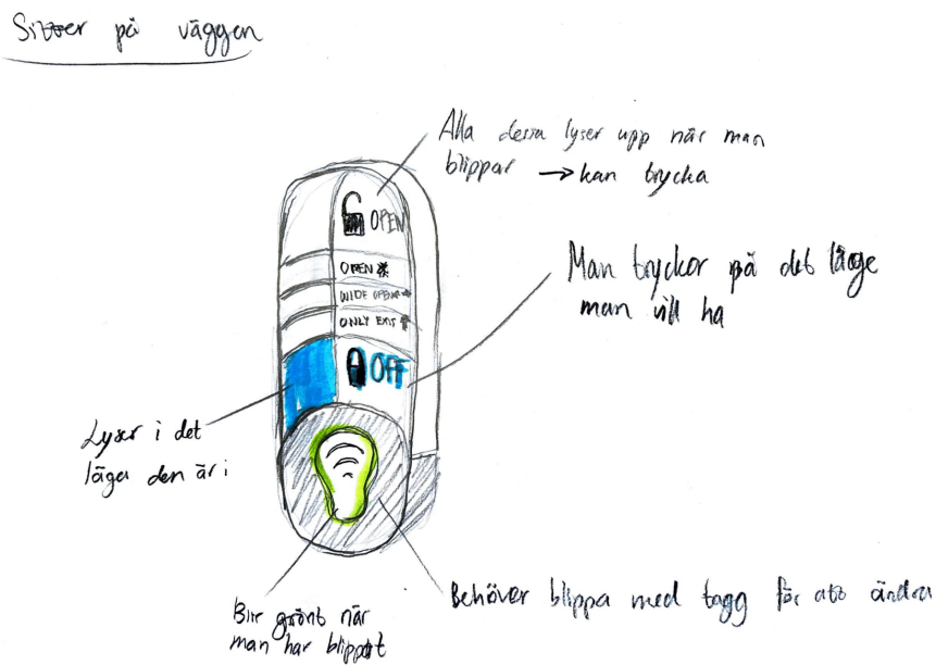
Figure 63: Buttons that lights up when pressed, tag activation.
