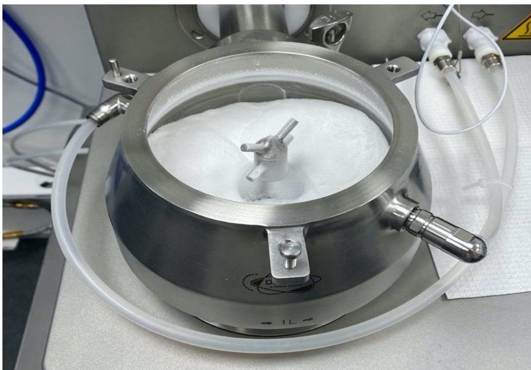
Figure 5: Picture of the Diosna mixing vessel. Some of the powder attached to the walls of the vessel was obtained for all batches.
