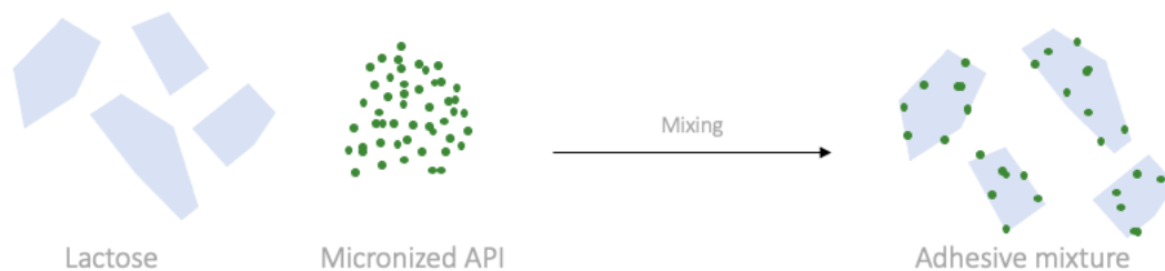
Figure 2: Schematic representation of lactose carrier particles and micronized API particles that, upon mixing, will create an adhesive mixture by which the finer API particles attach to the surfaces of the carrier particles. Figure adapted from [9].
