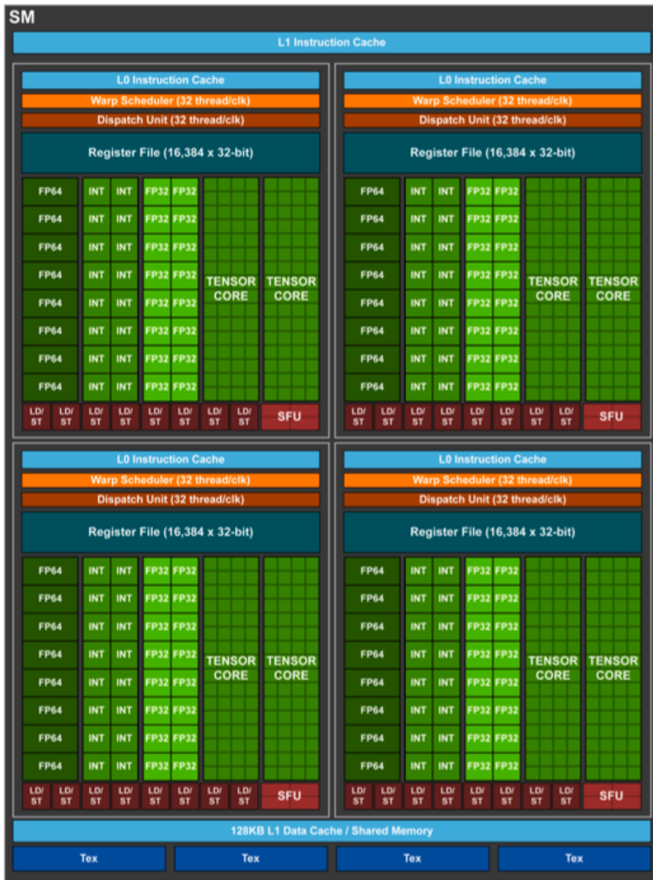
Figure 2.1: Nvidia SM with 4 processing blocks [2]
