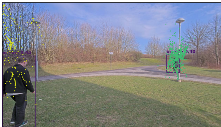
Figure 16: Combined image consisting of the YOLO annotation in Figure 14 and the projected clusters from Figure 15.
