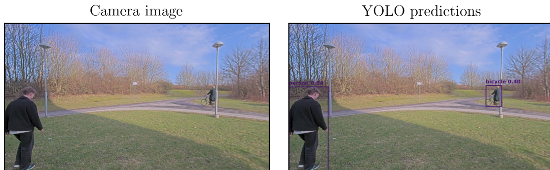
Figure 14: An example of a camera image from the data set, before and after YOLO-predictions are applied.
