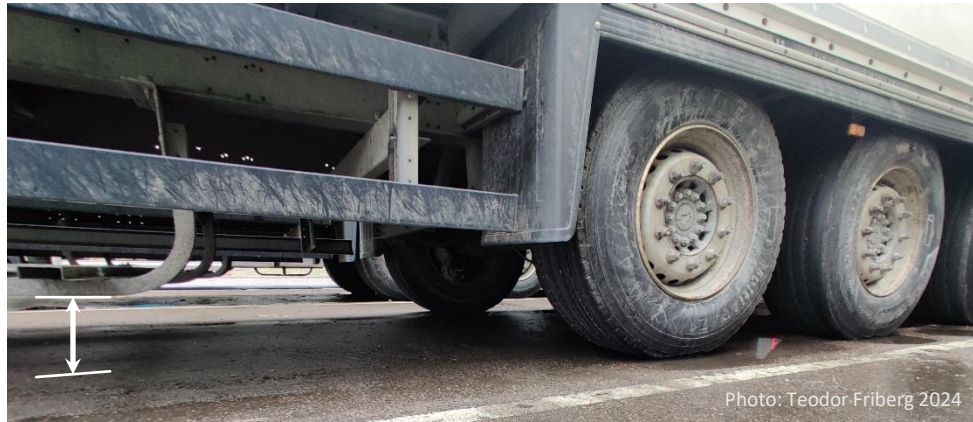
Figure 7.2 Truck clearance example. The arrow shows where the measurement was taken.
