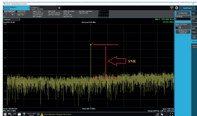
Figure 2.8: A screenshot of the UXA that shows the signal as a green dot in the middle and background noise (DANL) towards the bottom.
