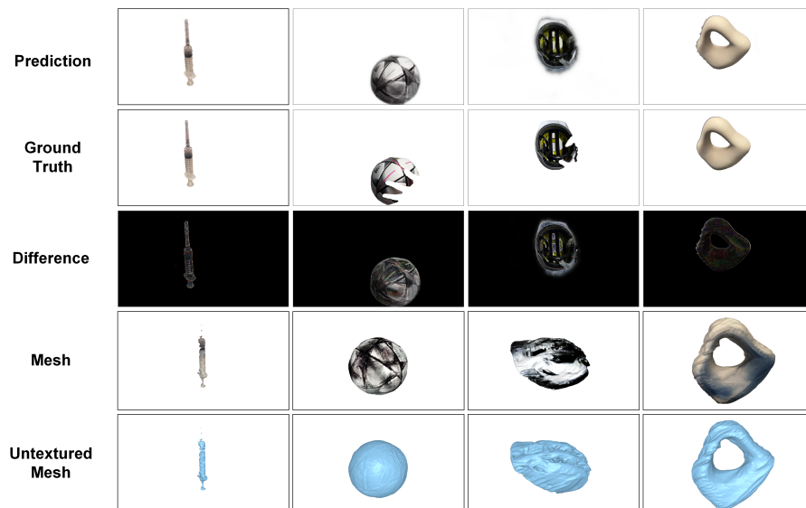
Figure 4.10: Reconstruction and rendering result on four objects. The football and helmet are captured by a static camera. The syringe and the statues are captured by the moving camera
