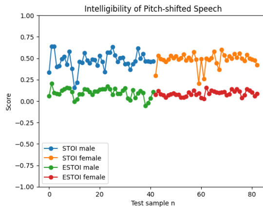
Figure 17: Speech intelligibility of Three-threaded Pitch Shifting on clean speech recordings from Data Set 1.
