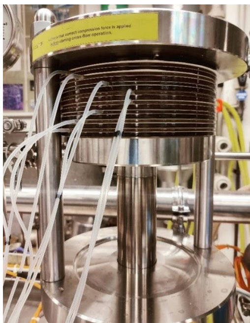
Figure 3.6. RO membranes in practice in the membrane house of M20 TestUnit, MemLab, Lund University
