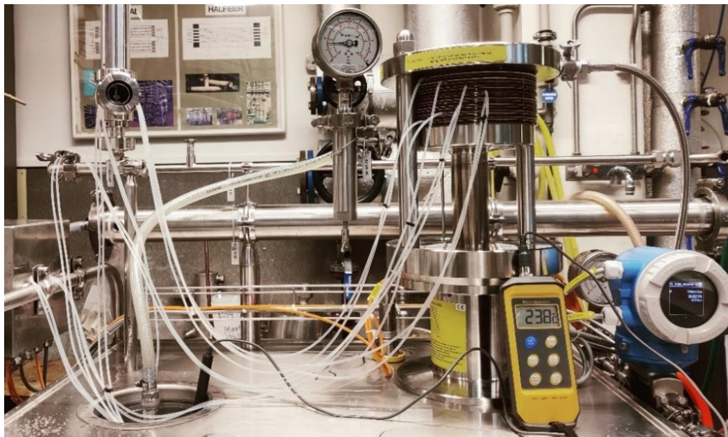
Figure 3.3. TestUnit M20 pilot system in performance during RO membrane filtration, Mem-Lab, Lund University
