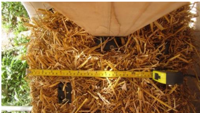
Figure 22: Location of inner and outer sensor in the straw bale wall (Marincioni & Bradshaw, 2023)
