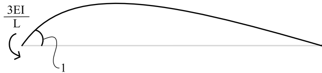
Figure 6.7: The elementary case that was used for calculating the spring stiffness in the modeled purlins.
