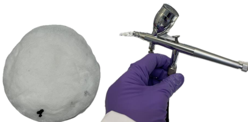
Figure 14. Treatment application onto cellulose sample through airbrush application.
