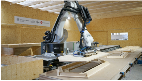
Figure 14: The heavy duty robot assembling a cassette _ source: (Institute for Computational Design and Construction, 2023)
