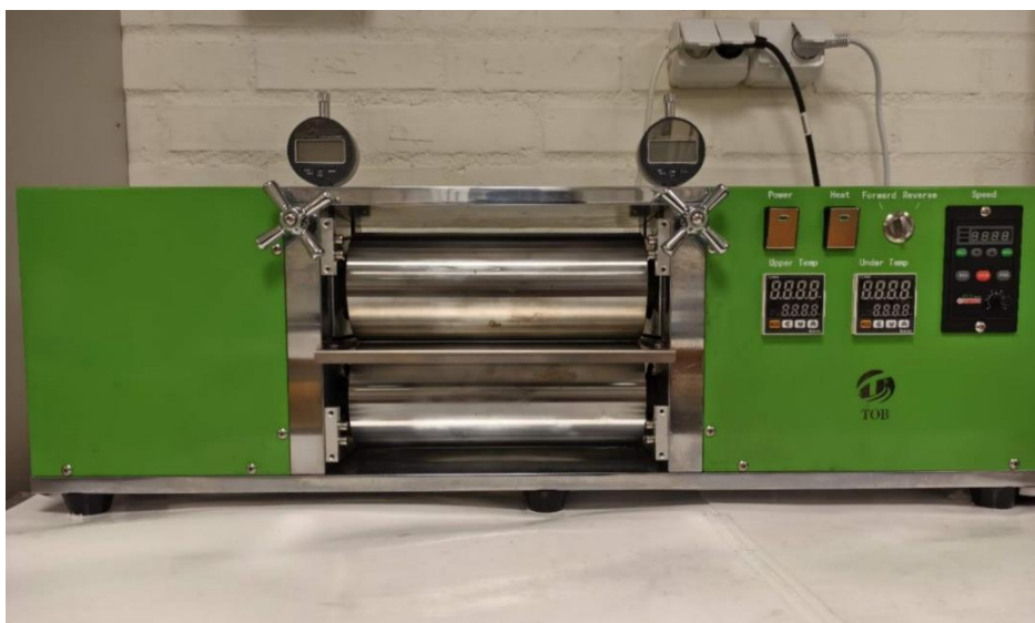
Figure 17: Roll-to-roll calendaring machine for dry coating method.
