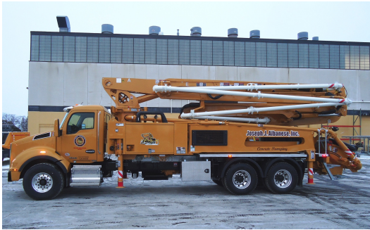
Figure 2.3: Example of a concrete boom truck type of device used to pour concrete, image by Joseph J. Albanese [7].
