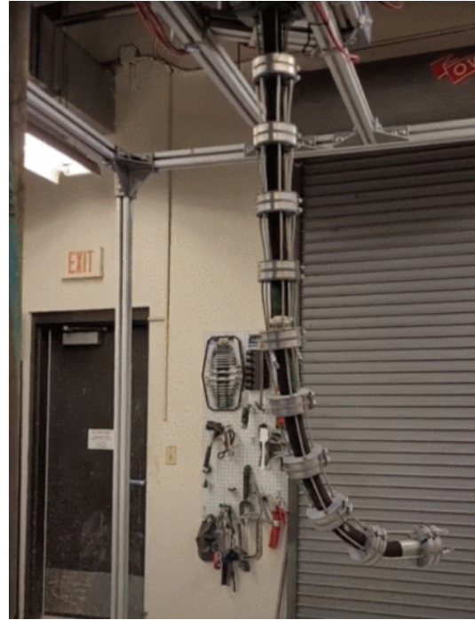
Figure 2.4: Prototype that achieves an automated tendon-driven motion of a flexible concrete house used for additive manufacturing, developed at Clemson University [8].
