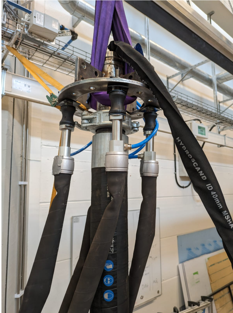
Figure 4.1: Top part of the prototype, highlighting the mounting points of the air muscles.
