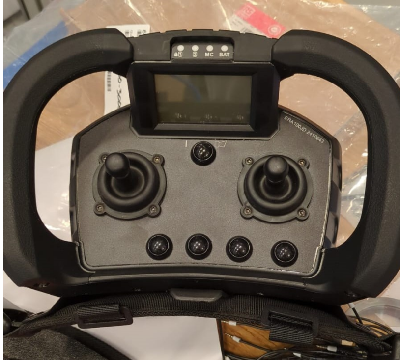
Figure 4.8: (6): Remote controller interface consisting of two joysticks, four programmable buttons and one button to initiate the wireless connection.
