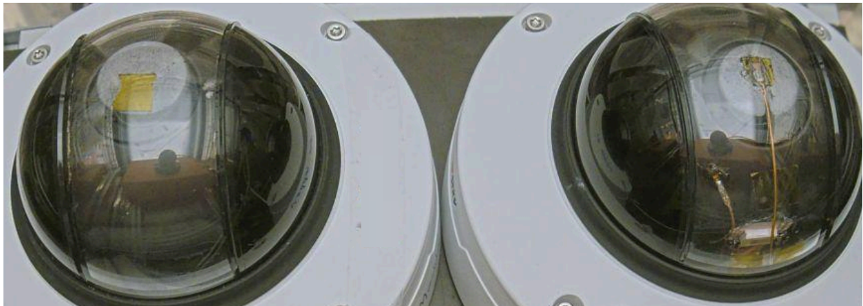
Figure 44: Image from the test, 32 minutes in. Condensation can be seen in both cameras as light circles in front of the optical FoV.
