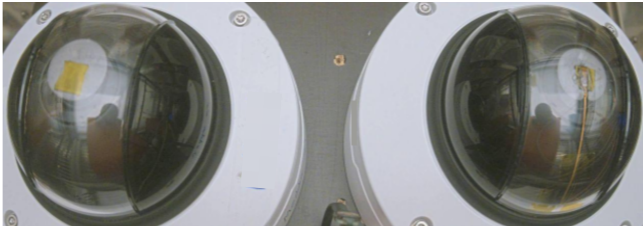
Figure 29: Image from test 2. Condensation can be seen in both cameras as light circles in the center of each dome.
