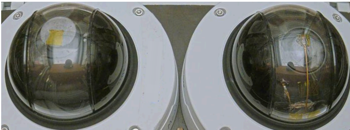
Figure 37: Image from test 6. Condensation can be seen in the left camera as a light circle in the center of the dome. A smaller, more transparent circle is visible in the center of the modified camera.
