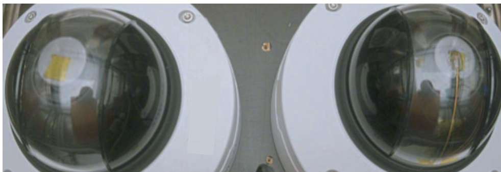
Figure 31: Image from test 3. Condensation can be seen in both cameras as light circles in the center of each dome.
