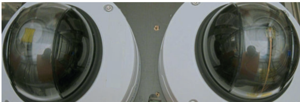
Figure 21: Image from test 3. Condensation can be seen in the left camera as a light circle in the center of the dome, while in the modified camera no condensation is formed.
