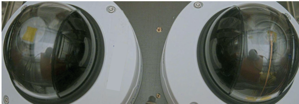
Figure 35: Image from test 5. Condensation can be seen in the left camera as light circles in the center of the dome. It is also possible to see a smaller, almost transparent circle in the center of the right camera.
