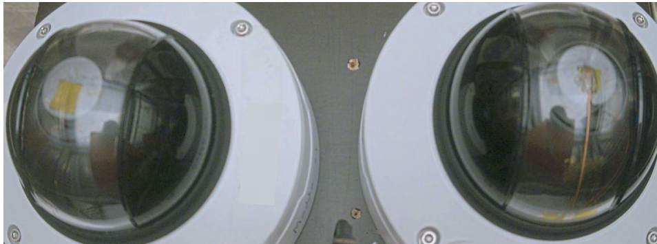
Figure 33: Image from test 4. Condensation can be seen in both cameras as light circles in the center of each dome.
