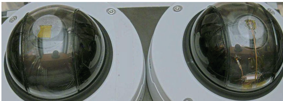
Figure 44: Image from the test, 32 minutes in. Condensation can be seen in both cameras as light circles in front of the optical FoV.
