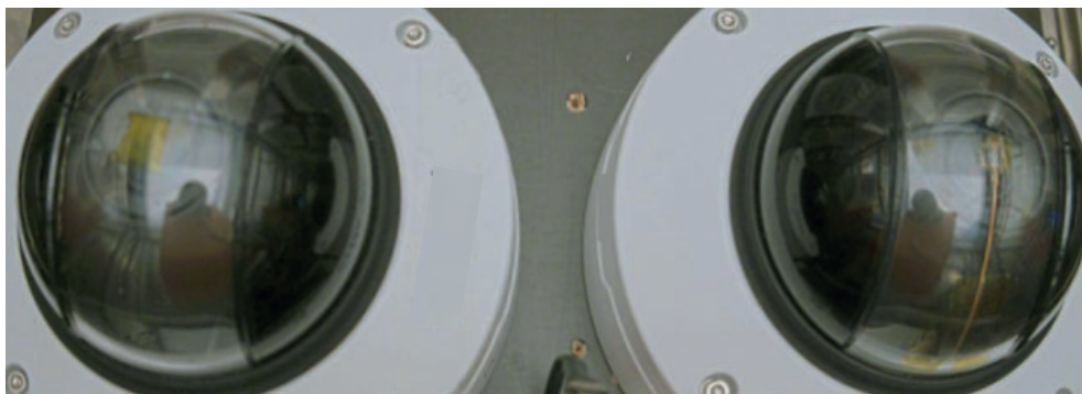
Figure 23: Image from test 4. Condensation can be seen in the left camera as a light circle in the center of the dome, while in the modified camera no condensation is formed.
