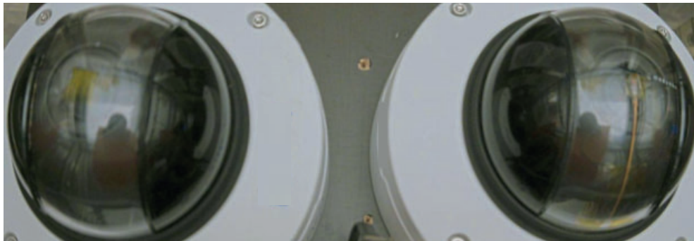
Figure 25: Image from test 5. Condensation can be seen in the left camera as light circles in the center of the dome, while in the modified camera no condensation is formed.
