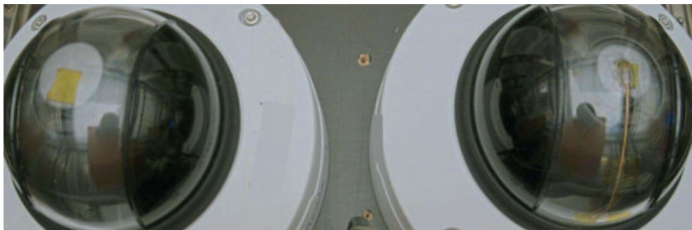
Figure 27: Image from test 1. Condensation can be seen in both cameras as light circles in the center of each dome.
