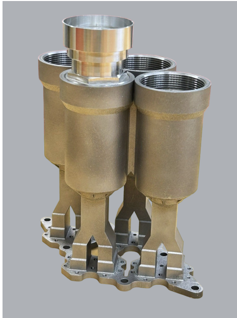
Figure 3.1: AM-SLM printed circularly polarized array antenna with a milled horn attached.
