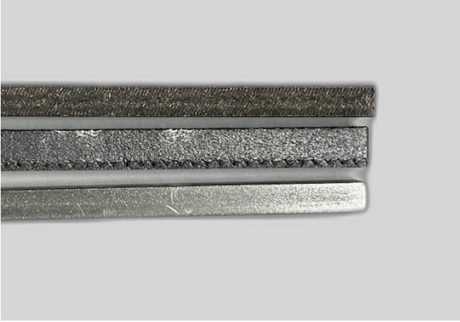
Figure 5.1: Metal samples for PIM test, from bottom: milled aluminum, AM-SLM vertical print, AM-SLM horizontal print.
