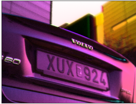
Figure 5.3: HSV image with H = \text{AoLP} , S = S_0 , and V = \text{DoLP} .
