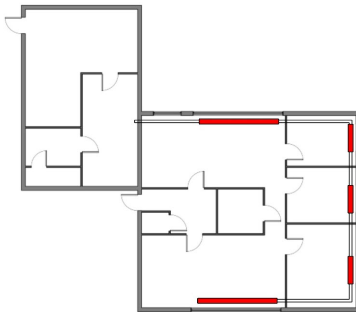
Figure 4.8 Layout of radiators and piping in Building 2. Rectangles marked in red are radiators, dual lines in between the radiators are the 2-way piping distribution.
