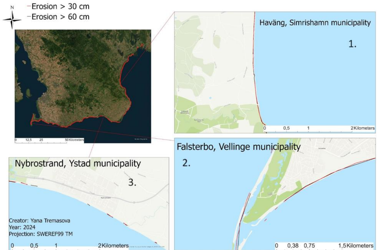
Figure 5: Map of Scania displaying areas where sediment eroded by > 0.3 m (red line) and > 0.6 m (black line), depicting three example areas of Simrishamn, Vellinge, and Ystad municipalities as zoomed in illustrations.
