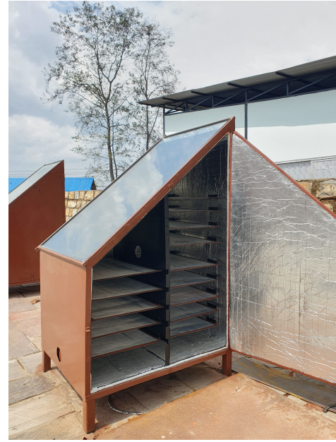
Figure 4: Third generation dryer (picture by Magnus Lundquist). See Appendix G for cost calculations.
