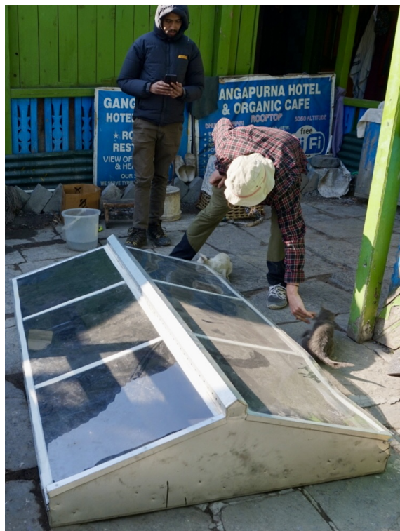
Figure 11: Direct solar dryer used in Pisang, Manang. Picture by Ida Sonesson.
