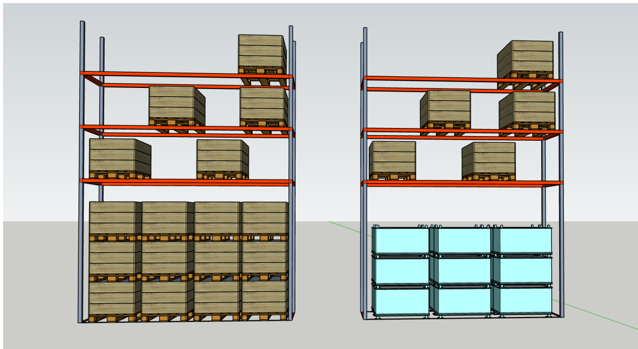
Figure 6.6: A M1-rack with fully utilized floor storage, and some SKUs on upper levels.
