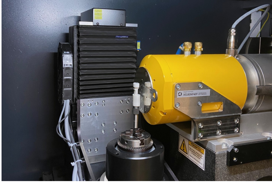
Figure 7: Setup with samples in the industrial nanofocused X-ray CT-scanner Phoenix Nanotome, available at Tetra Pak in Lund.
