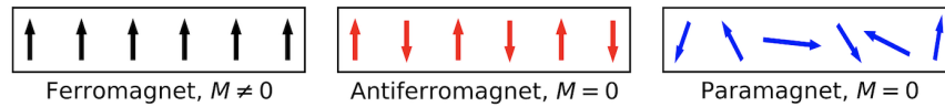
Figure 1: Alignment of localized atomic magnetic moments at low temperatures and in the absence of an external magnetic field. The observed magnetization is M .
