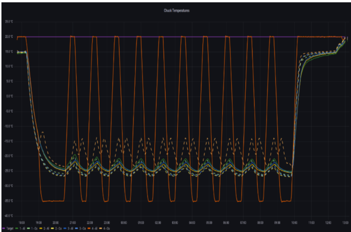
Figure 5.1. Temperature recorded during the thermal cycle performed on the 9th of April. The dashed lines indicate the temperature measured in the copper part of the chuck. The dotted lines indicate the temperature in the aluminum. The temperatures on chuck number four are plotted in orange.
