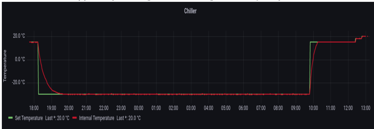
(b) Chiller temperature during the thermal cycle sequence.
