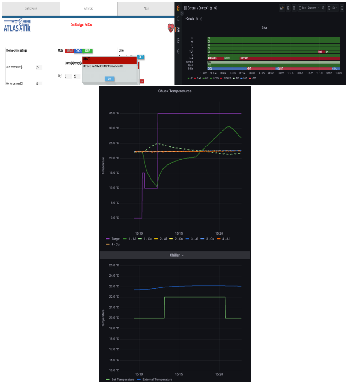
Figure 15: Interlock firing (top), temperature taking corrective action (bottom), as intended.
