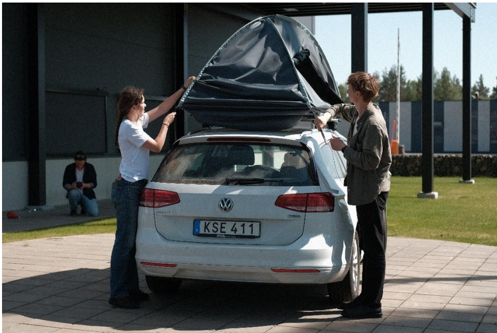
Figure 53: Tent is pitched by pushing the tent poles into the grooves. (Source: Authors' own work)
