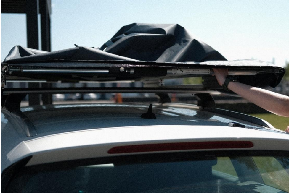
Figure 52: Base fabric is stretched to achieve a flat sleeping surface. (Source: Authors' own work)
