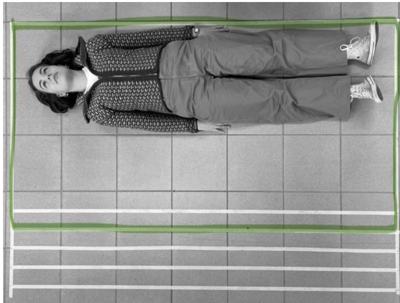
Figure 14: Bed size test with a single person as test subject, the test was carried out with two test subjects at a time. (Source: Authors' own work)
