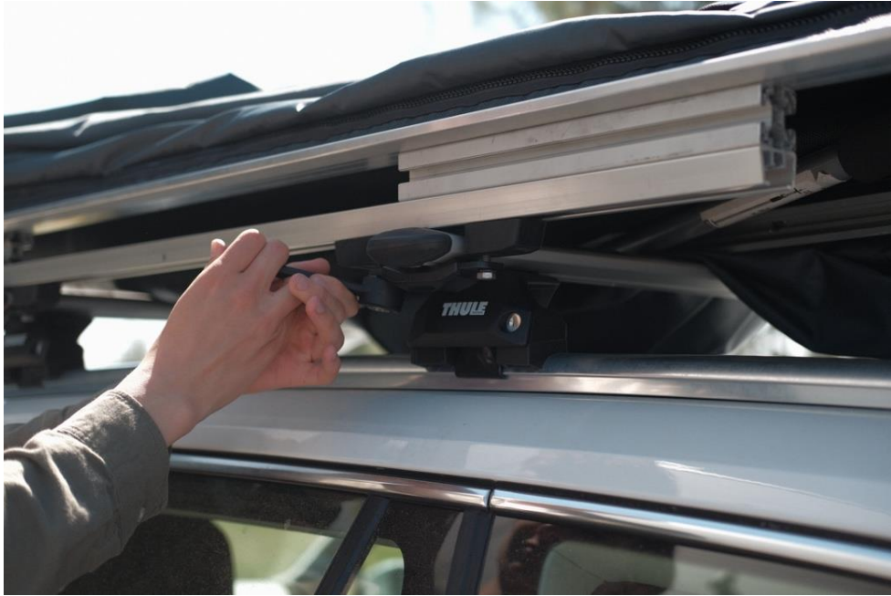
Figure 48: A long side is secured to roof racks. (Source: Authors' own work)
