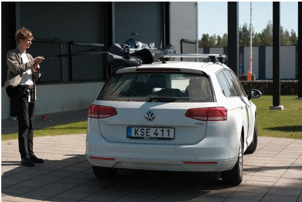
Figure 61: Straps are used to slide the long side together; the tent is now in transport mode. (Source: Authors' own work)
