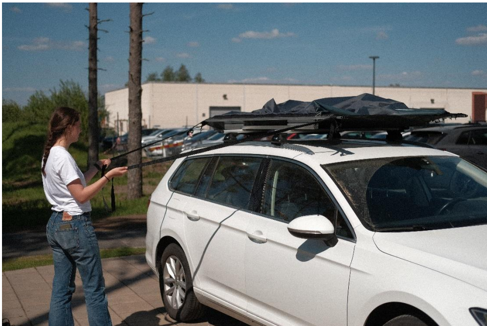
Figure 51: Straps are pulled to slide out the bed. (Source: Authors' own work)
