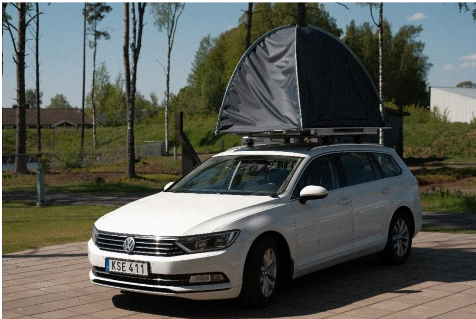
Figure 55: The ultra-lightweight RTT prototype, pitched. (Source: Authors' own work)
