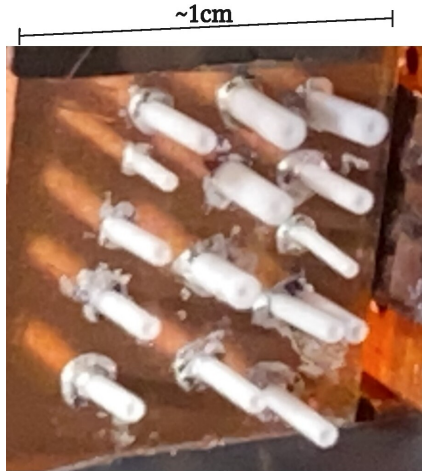
FIG. 1: Example of several samples mounted on a single holder for an ARPES experiment. Each crystal (not fully visible) is glued onto a copper plate together with a ceramic rod which facilitates cleaving inside a vacuum chamber. By pushing the rods, the crystals cleave and a pristine surface is exposed within the vacuum environment. The cleaving process does not always produce useful surfaces, often necessitating multiple attempts. The figure shows an example of a particularly difficult case, where 15 identical crystals were mounted on a single holder.
