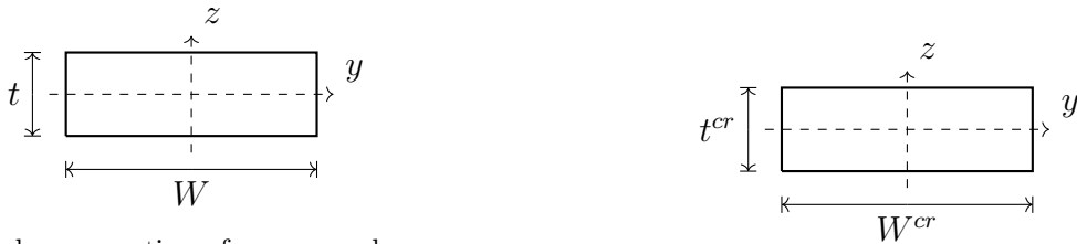
(a) Initial cross section of noncreased paperboard beam segments ab and cd , assigned the same thickness and width as the paperboard in the continuum approximation.
