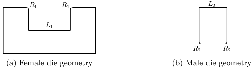
Figure 4: Female- and male die tool geometries with relevant geometric parameters marked out.
