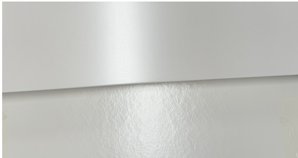
Figure 4.17: Fiber raising front A (60/95)
