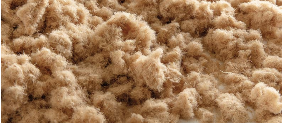
Figure 2.5: Wood fibers used for MDF [4]
