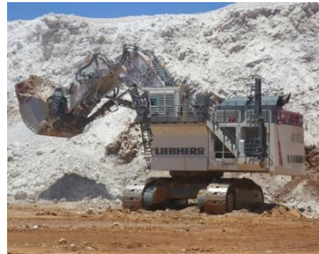
Figure 2: Face Shovel Equipment Configuration (Liebherr-International Deutschland GmbH, n.d.)
