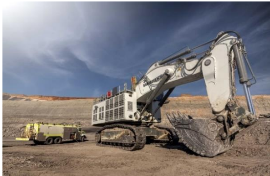
Figure 1: Backhoe Equipment Configuration (Liebherr-International Deutschland GmbH, n.d.)
