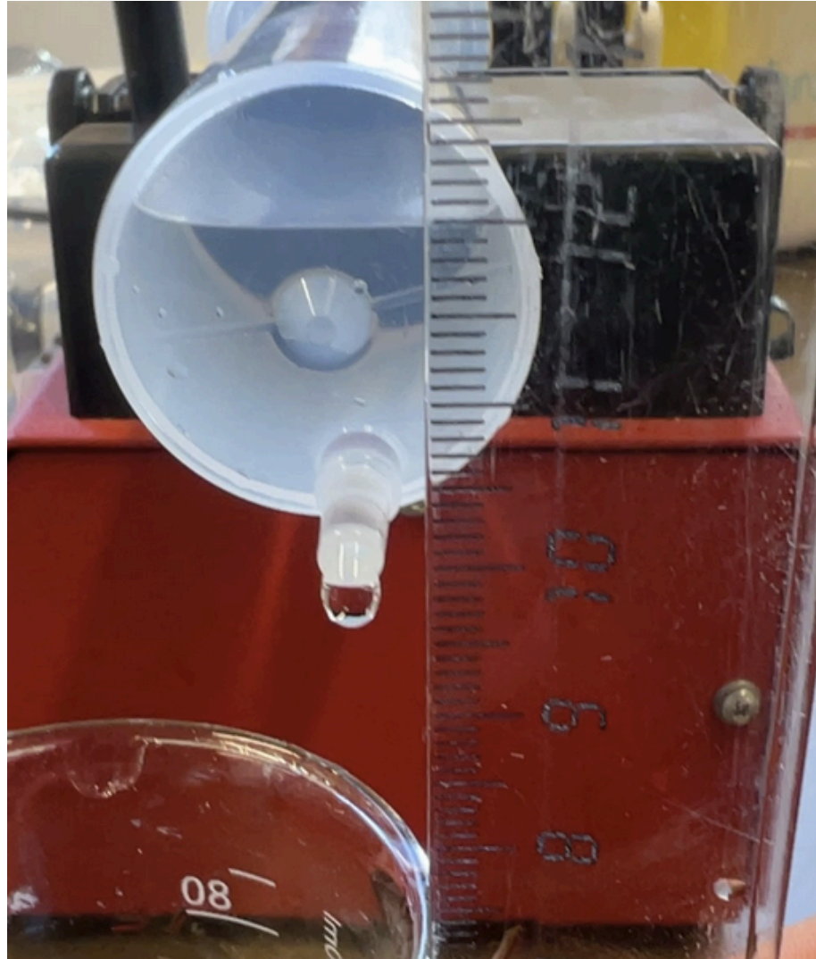
Figure 3: Droplet measuring technique (aiming for large size, 5mm droplet)
