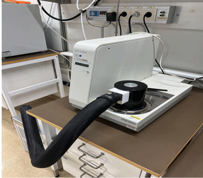
Figure 5: Differential Scanning Calorimeter Model 6200 from SEIKO Available at Division of Food and Pharma
