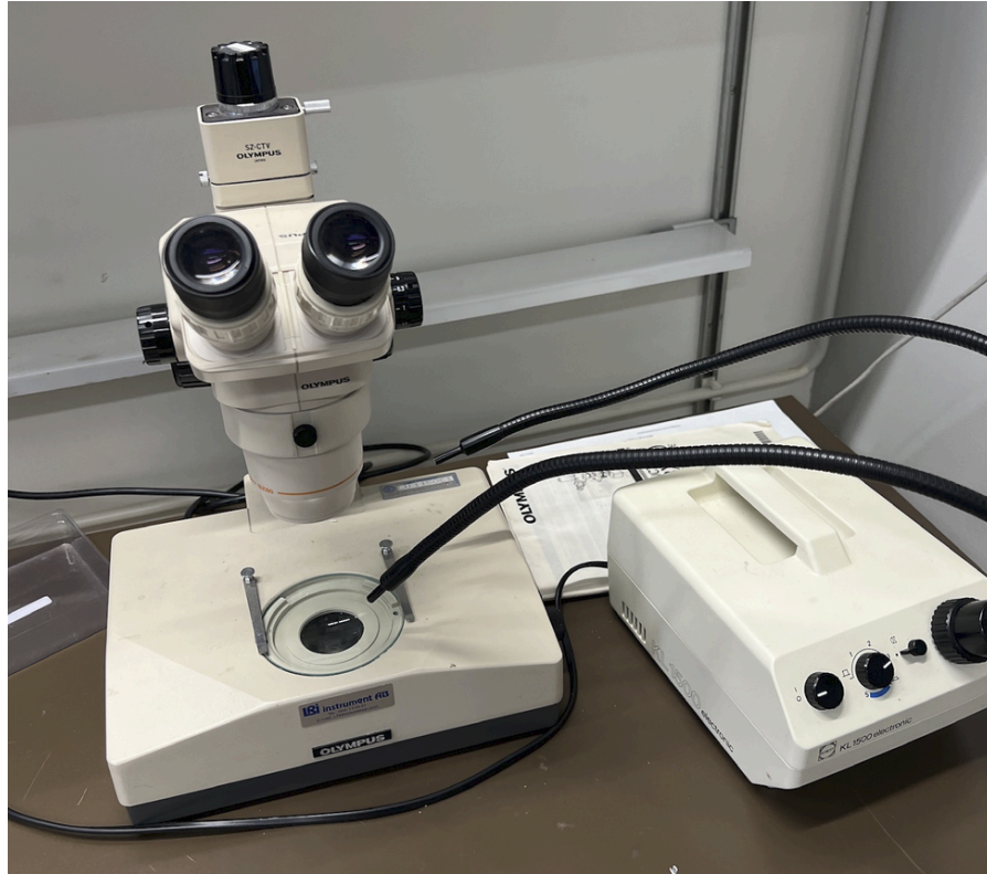
Figure 10: Stereo microscope available at Division of Food and Pharma with SCHOTT light source
