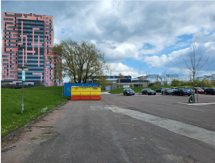
Figure 3.10: Field of view from the location of the radar for the measurements of the different scenes. The antennas are to the best of the operators ability directed so that the bore-sight is in the center of the closest container, determined to be at a range of 24.5 m by the use of measuring tape.
