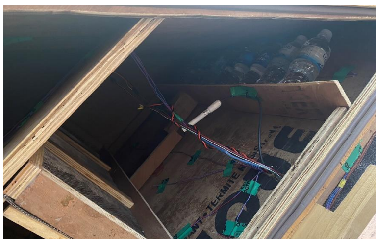
Figure 3-9: Heat storage inside dryer
