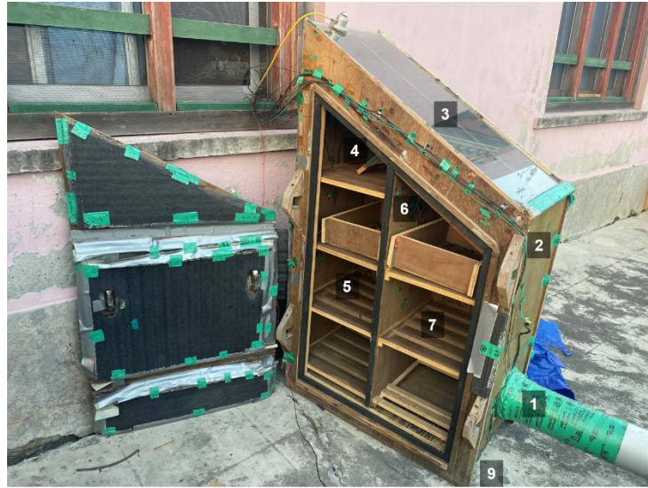
Figure 2-2: Photo of dryer's initial design in Bhutan
