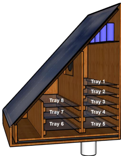
Figure 3-4: Tray arrangement inside dryer
