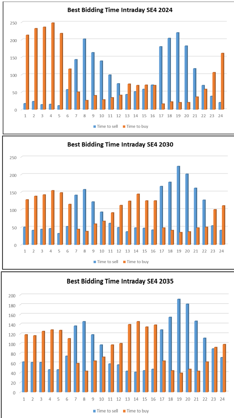
Figure 37 The costliest and cheapest Elbas hours of a day for bidding zone SE4 in 2024, 2030 and 2035
