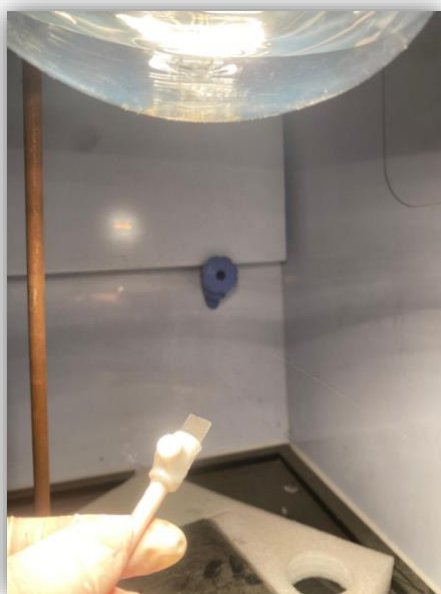
Figure 8- Drying of carbon paper with the catalys
