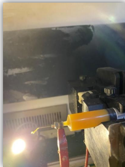
Figure 6- Prepared polymer inside of sirynges ready for electrospinning
