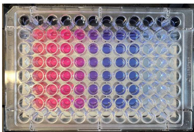
Figure 127. Image of a 96-well plate after a 10 min resazurin assay. Column 2, with the highest cell concentration (OD 1.2), shows the most color change, indicating high metabolic activity. Contrastingly, column 8, with the lowest cell concentration (OD 0.1), displays minimal color change. The gradient of color from left to right reflects decreasing cell concentration and metabolic activities. Column 9 is the control containing only resazurin, showing the baseline color.
