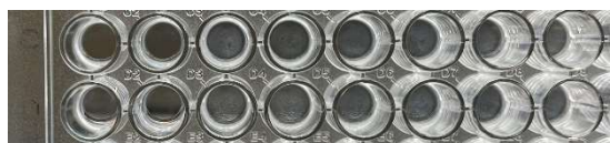
Figure 6. Image of a 96-well plate (Plate 1) after washing test plate where C1-C2 has been washed one time with saline, and D1-D2 washed one time with DPBS.
