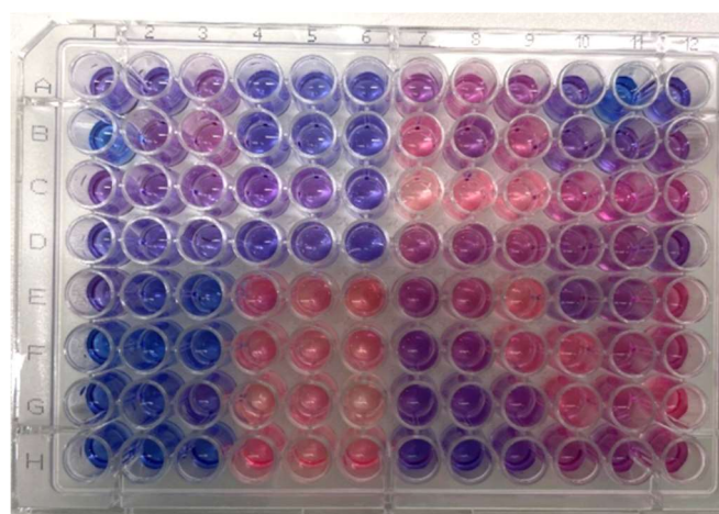
Figure 7 2. Image of a 96-well plate after resazurin staining, showing cell viability after 24 h of enzyme treatment and 40 min of incubation with resazurin. The enzyme concentrations decrease from top to bottom, and the wells are organized as follows: Nuclease I (A1:D3), Lysozyme I (A4:D6), Protease I (A7:D9), Protease II (A10:D12), Enzyme tablet (E1:H3), Protease III (E4:H6), Protease IV (E7:H9), and Anti-acneic peptide (E10:H12). The color ranges from blue, indicating low cell viability, to light pink, indicating high cell viability.
