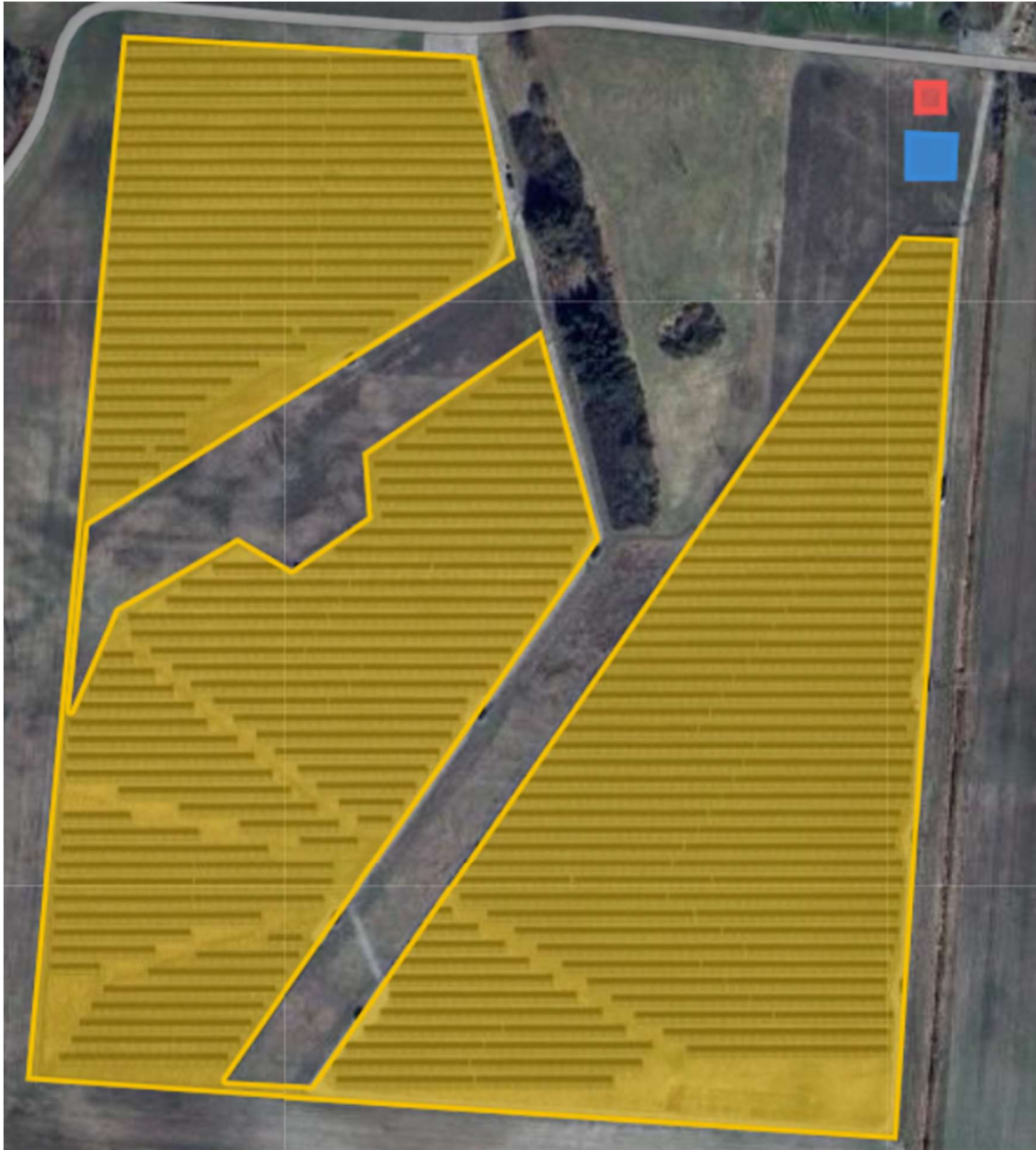
Figure 38 Space requirement for 18MW Skurup solar farm with BESS installation, red square: BESS installation for energy shifting, blue square: BESS installation for constant power, yellow area: solar farm (MyMaps, Google)
