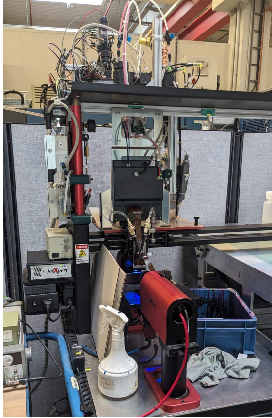
Figure 4.3: Picture of the experimental setup, showing the dropwatcher installation.
