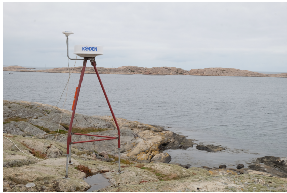
Figure 3.5: The radar used to capture the boat passages.
