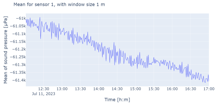
(b) The mean sound pressure using 1 minute subwindows for sensor 1.
