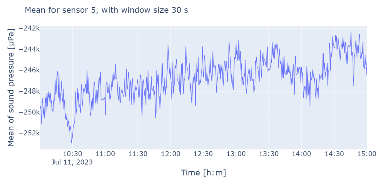
(a) The average sound pressure using 30 second subwindows for sensor 5.
