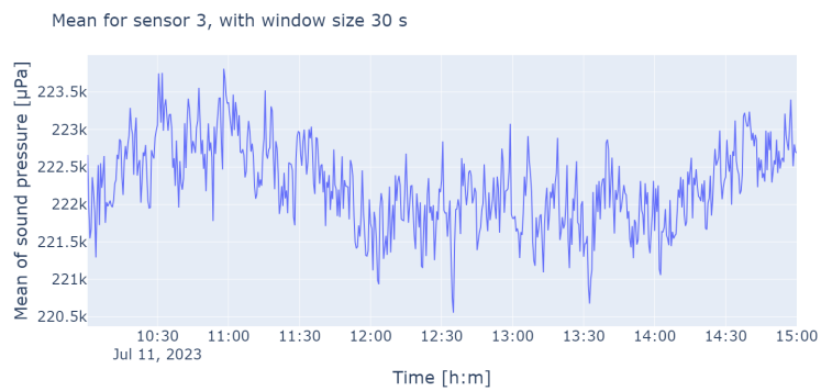
(a) The mean sound pressure using 30 seconds subwindows for sensor 3.
