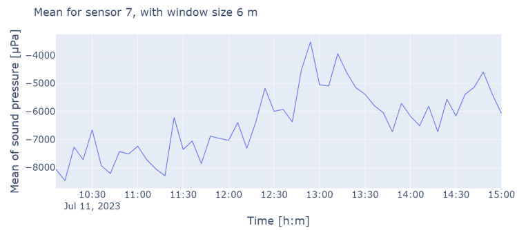
(e) The mean sound pressure using 6 minutes subwindows for sensor 7.
