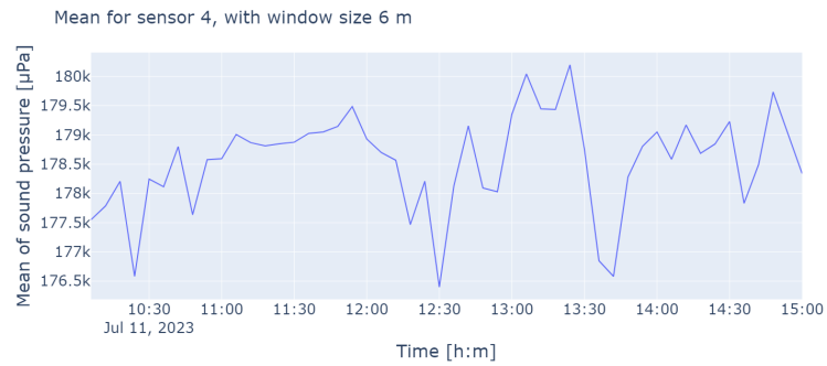
(e) The mean sound pressure using 6 minutes subwindows for sensor 4.
