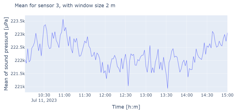
(c) The mean sound pressure using 2 minutes subwindows for sensor 3.
