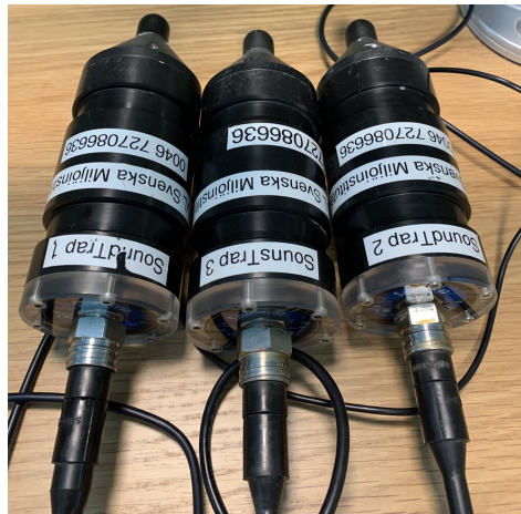
Figure 3.2: The three Soundtrap loggers used to measure the underwater noise.
