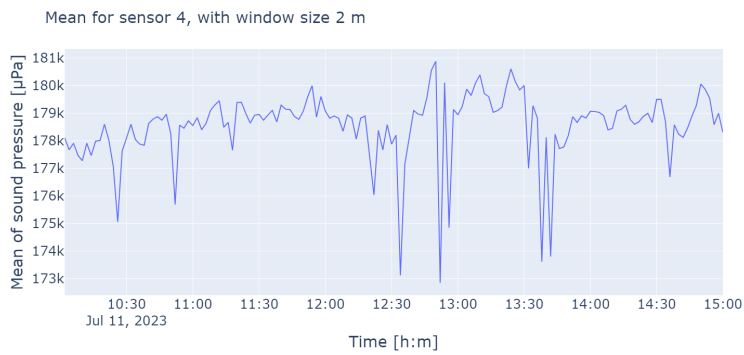
(c) The mean sound pressure using 2 minutes subwindows for sensor 4.
