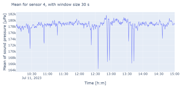
(a) The mean sound pressure using 30 seconds subwindows for sensor 4.
