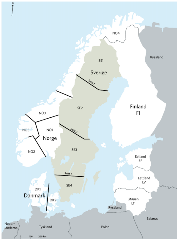
FIGURE 2.2: Illustration of the four Swedish bidding zones, received through email contact with the Swedish TSO (Svenska Kraftnät).
