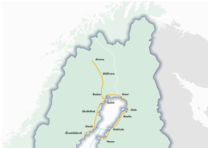
FIGURE 2.8: Illustration of the preliminary hydrogen pipelines in the Bothnian Bay, picture from Nordic Hydrogen Route [35].
