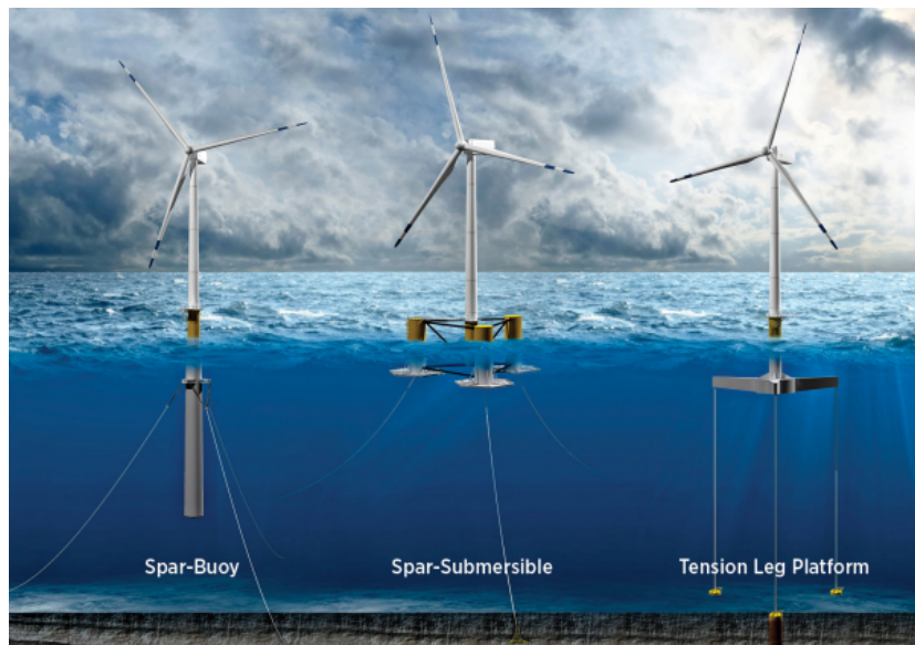
Figure 3.7: Illustration of three different floating wind power foundation concepts.
