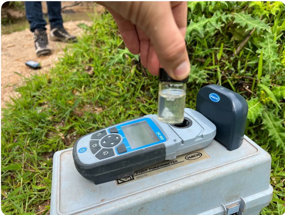
Figure 3.14 Measuring turbidity in situ (Nyagako sub-catchment).
