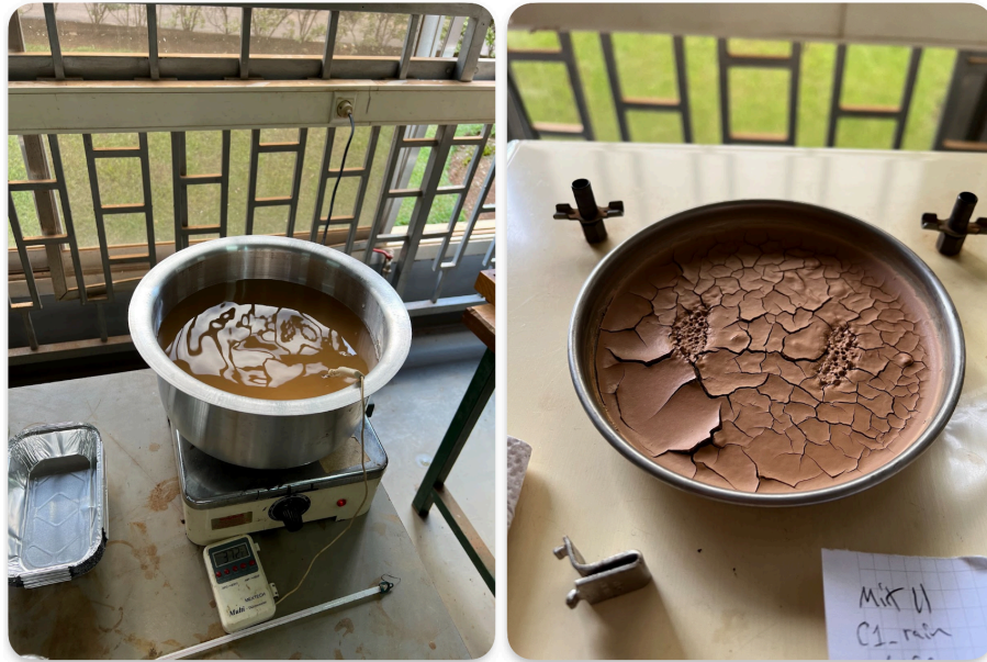
Figure 3.11 Left: Evaporation of sediment sample. Right: Evaporated sediment sample.
