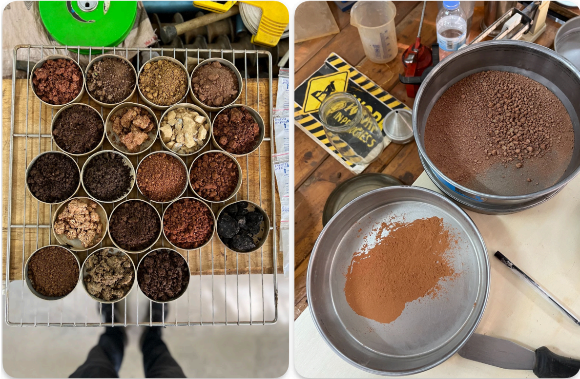
Figure 3.10 Left: Air-dried soil samples. Right: Sieved soil samples through < 63 µm pore size.
