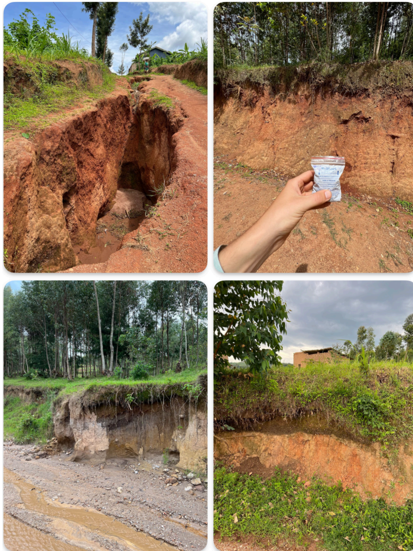
Figure 3.8 Top left: Gully where a soil sample was collected. Top right: Collected soil sample in zip bag from excavated land. Bottom left: Channel bank where a soil sample was collected. Bottom right: Both top and subsoil illustrated.
